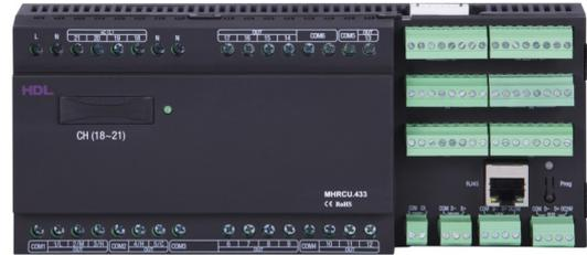
**HDL-MHRCU.433** 22CH Mix Controller is a module which with gateway function, it has mix controller, 22 channel outputs, 24-channel dry contacts and 12-channel LED outputs.
